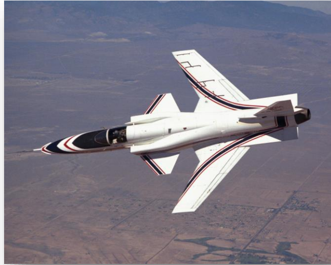
The Grumman X-29, an experimental forward-swept-wing aircraft used in NASA research. The aircraft achieved a high degree of maneuverability from its inherent instability. Feedback control was used to keep the plane flying properly. Photo Credit: NASA
